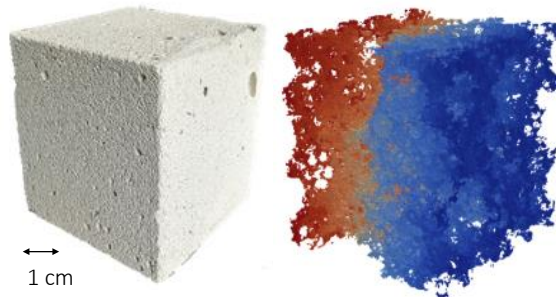
Figure 3: Typical concrete foam and 3D heat flow schematization.
