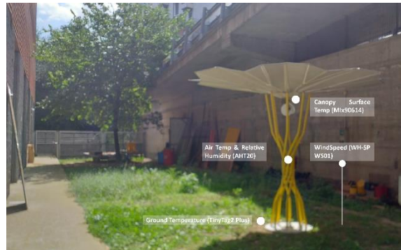
Figure 2 | Canopy installation and sensor set up at test site
