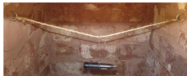
Figure 5: The loggers inside the test cells during monitoring.
