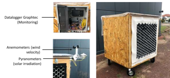
Figure 4: Photograph of some of the sensors and of the prototype integrated to a test box in real climate conditions.
