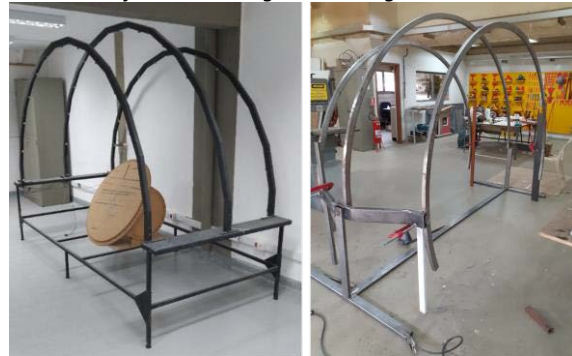
Figure 4: Heliodon before and during remodelling.
