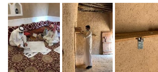
Figure 1: HOBO loggers installed in vernacular houses
