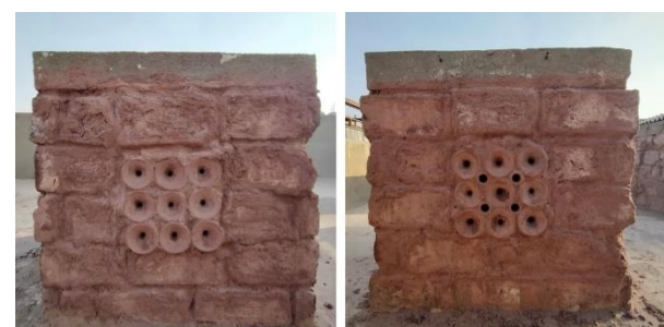
Figure 4: The eco-cooler after completing the drying process and before monitoring started.
