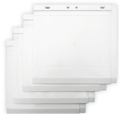
Figure 4: Recycled HDPE films obtained by injection
