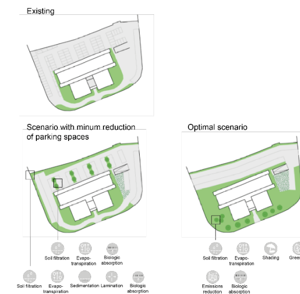
Figure 5: Two scenarios of application of NbS in a parking lot: the first one introduces drain ditches to collect rainwater, the second one is an optimized version that improves temperature regulation and the quality of the area.
