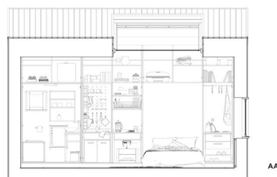
Figure 6: Cross section of the house showing the different interior foldable facilities.
