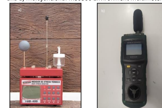
Figure 5: Used Equipment: a) stress meter (TGD-400 Instrutherm) and b) Multifunctional MS6300 Environment Multimeter
