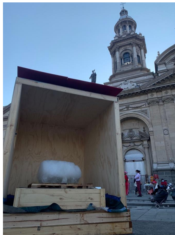
Figure 6: Local regulations box with the ice inside after 10 days (230 kg of ice). Source: Authors.
