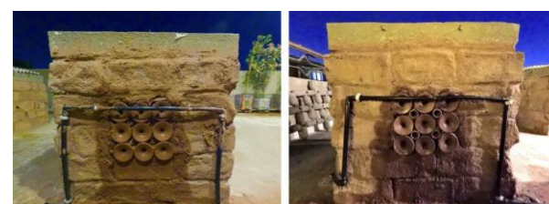
Figure 6: The test cells in the evening after the water sprinkling for evaporative cooling.
