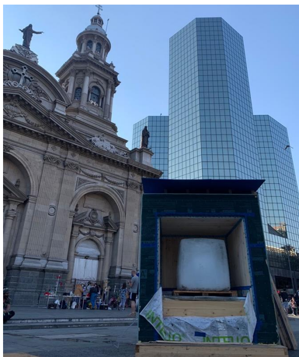
Figure 5: Passivhaus box with the ice inside after 10 days (645 kg of ice). Source: Authors.
