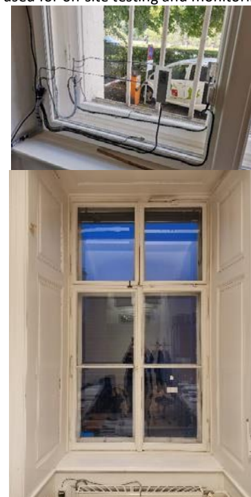
Figure 5: Two of the vacuum-glass equipped casement windows used for on-site testing and monitoring.
