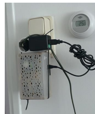
Figure 1: The monitoring boxes installed in the dwellings, developed by industrial partner OfficeVitae.
