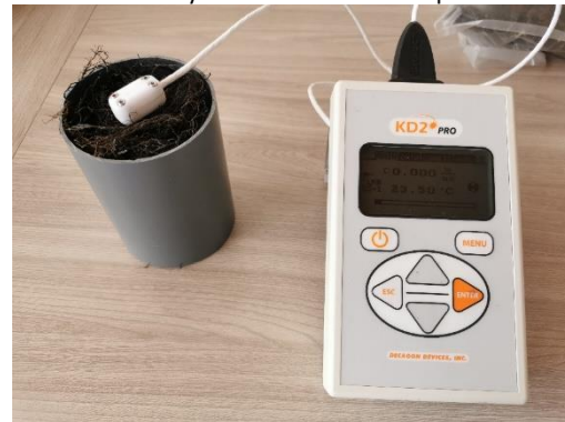
Figure 2: Thermal conductivity measurement of samples.
