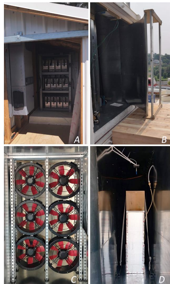
Figure 4: Photos taken during construction and commissioning of the chamber. A- doghouse interior, B- removable fairing on the door side. C- fan array facing the supply side. D- 1:3 prototype model placed in the test side.
