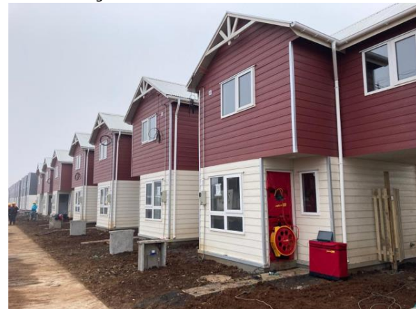
Figure 3: Blower Door test of a house in Labranza complex, Temuco, La Araucanía Region.
