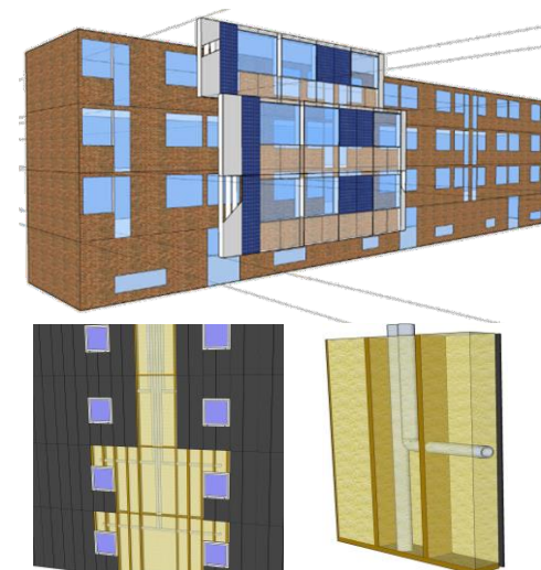
Figure 1. Concept visualization of the prefabricated façade modules, including added insulation, supply air ducts, and heat recovery.
